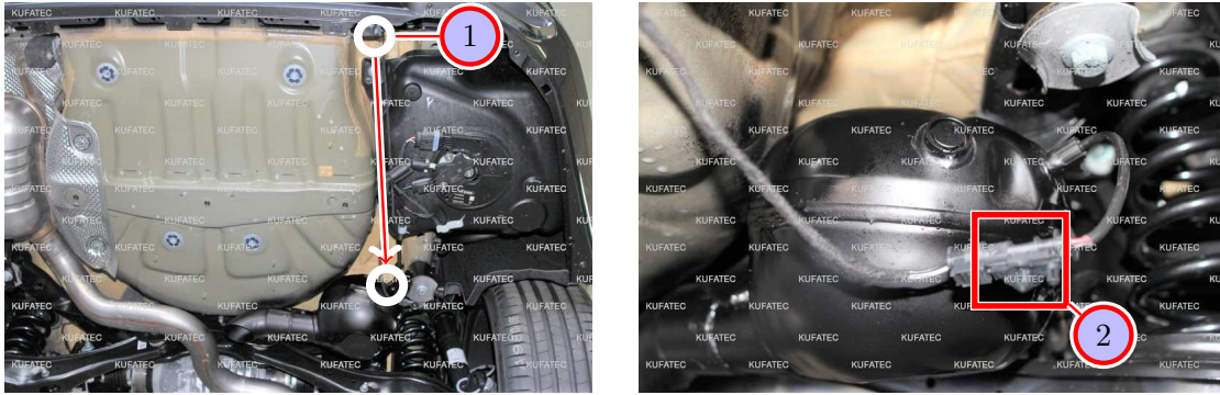
Figure 10: Cable routing to the sound generator
