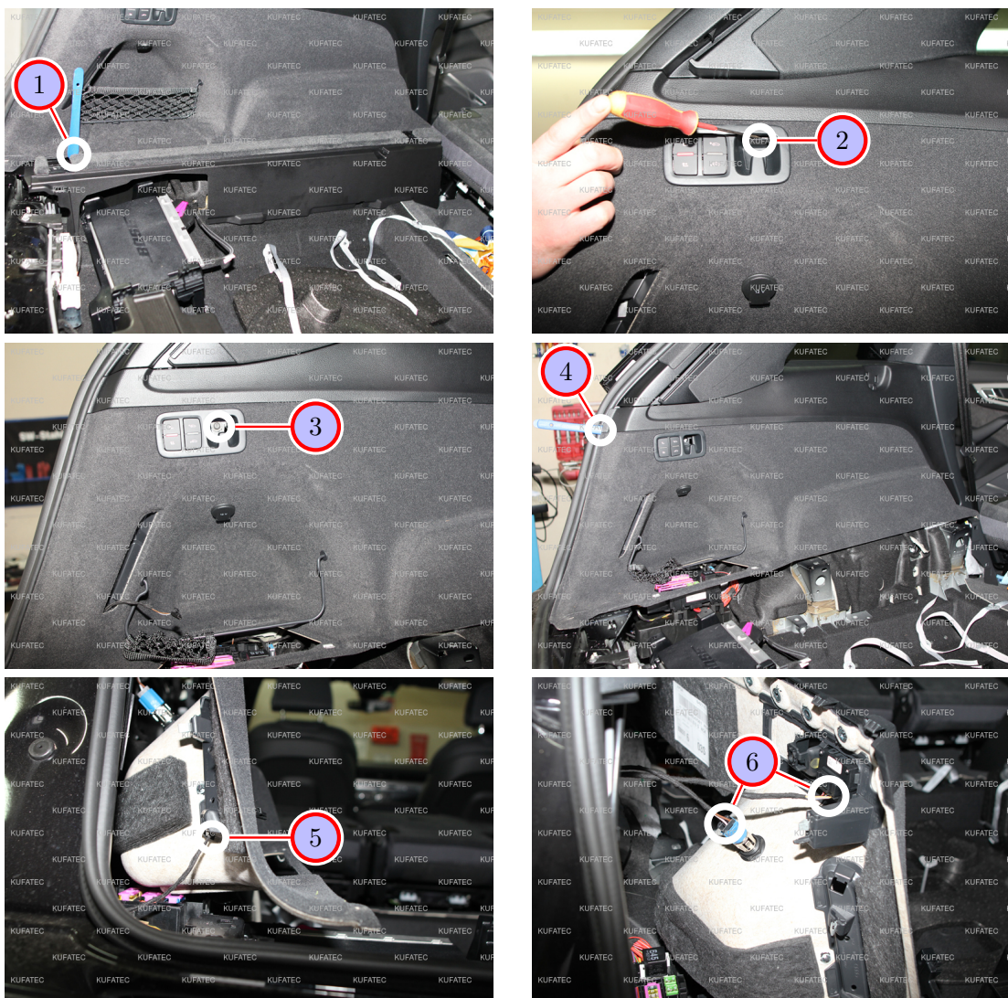
Figure 5: Disassembly left side covering trunk
