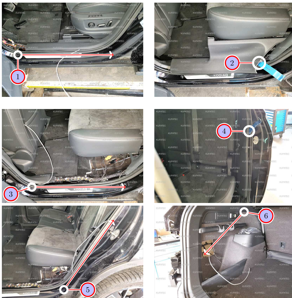
Figure 7: Cable routing to the sound generator
