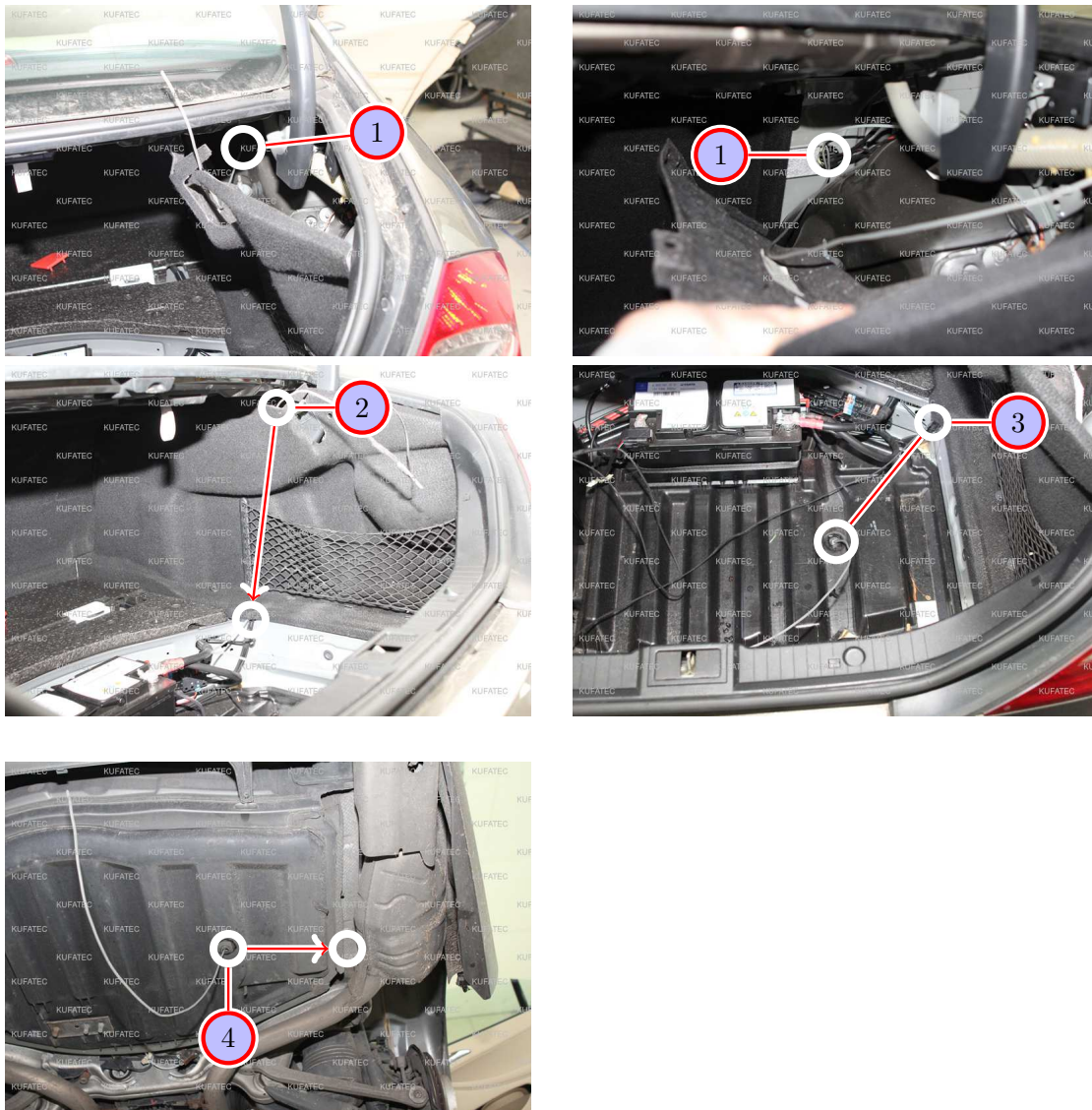
Figure 12: Cable routing to the underbody
