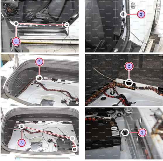
Figure 9: Routing connecting cable sound generator
