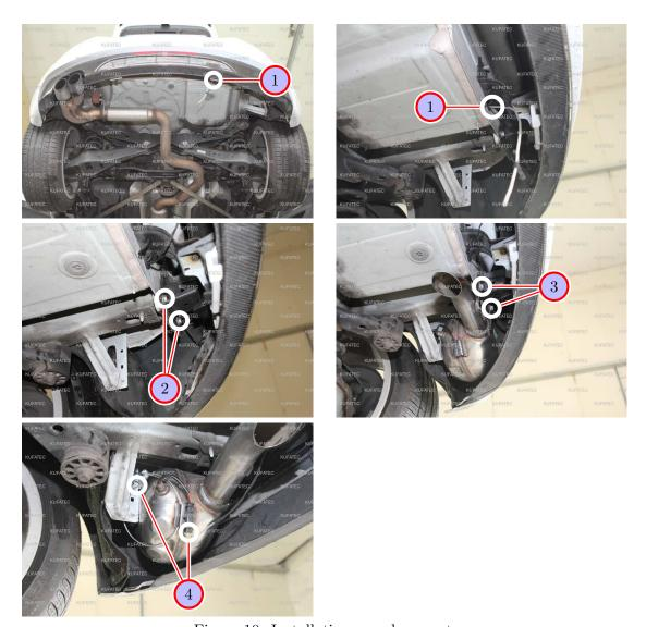
Figure 10: Installation sound generator
